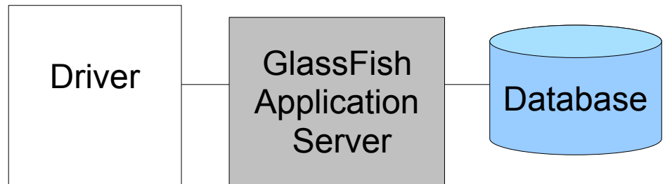
Figure 1. Typical benchmarking setup with driver, SUT and DB on separate machines.
